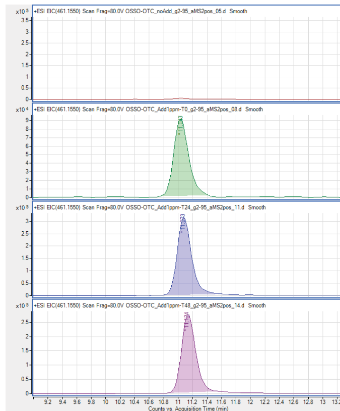
Fig. (3). From the top, ESI(+)-MS EIC of m/z 461.155 ion shown in the retention window of bone with OTC non-spiked at 0, 24 and 48h.
